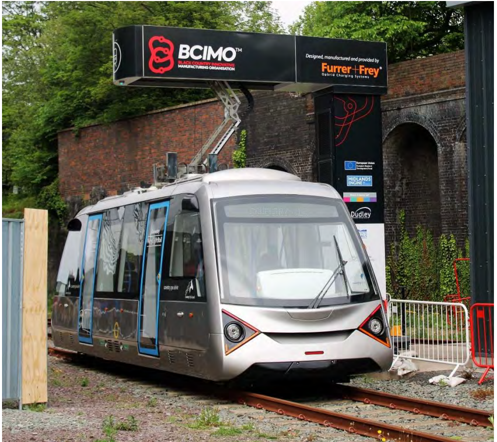
above VLR being under the charging arch 17.05.25 (Aidan Turner)
