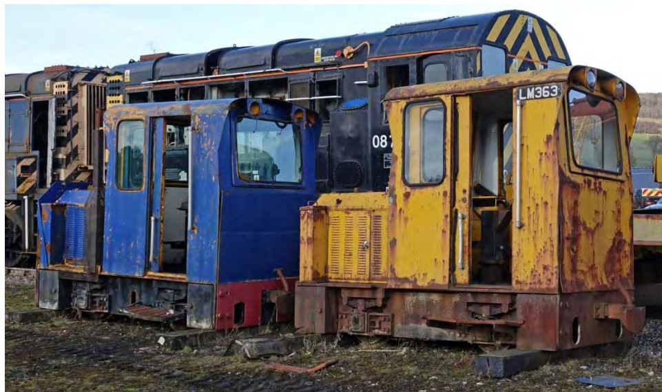
left & below examples of the Dundalk Works built 4wDH locos, LM 363 & LM 370, Wolsingham these locos were previously used on a contract for the Manx Electric Rly, IoM before arriving at WEA in January 2011
