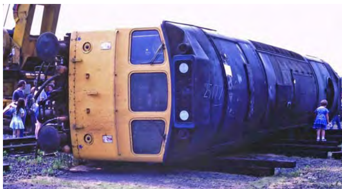
25177 (D7527): built 01/65 w/d 11/82 was then used for accident tests, firstly at Stratford Open Day 9 th July 1983 as seen above by Doug Slater, where tipped over to demonstrate lifting by the resident crane, then to Temple Mills Yard for re-railing exercise on the 26 th March 1984 before returning to Stratford from where it headed to Reading via a breakdown test on the 5 th June 1984
