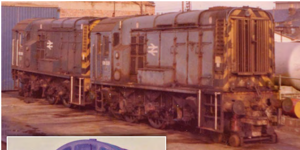
above 08639 + 08398 awaiting onward movement to Swindon Works with coupling rods removed and both appear to be missing an axle so jacked up on wheel skates, Gloucester Horton Road Depot, 19 th February 1977 (Andy Jones)
