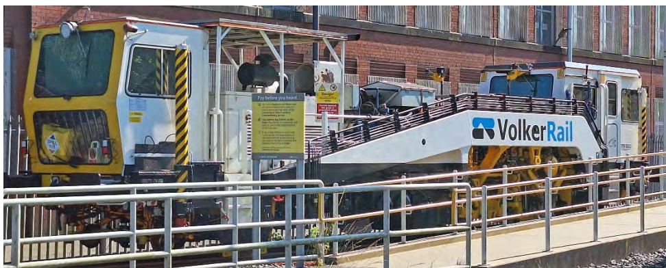
right & below Plasser & Theurer Beaver 90/4 ZW Tamper TPB 51002 99.70.9908.008-4 operated by Volker Rail Shaw & Crompton, Manchester (13.30) 18 th September 2024 (Harold Hull)
