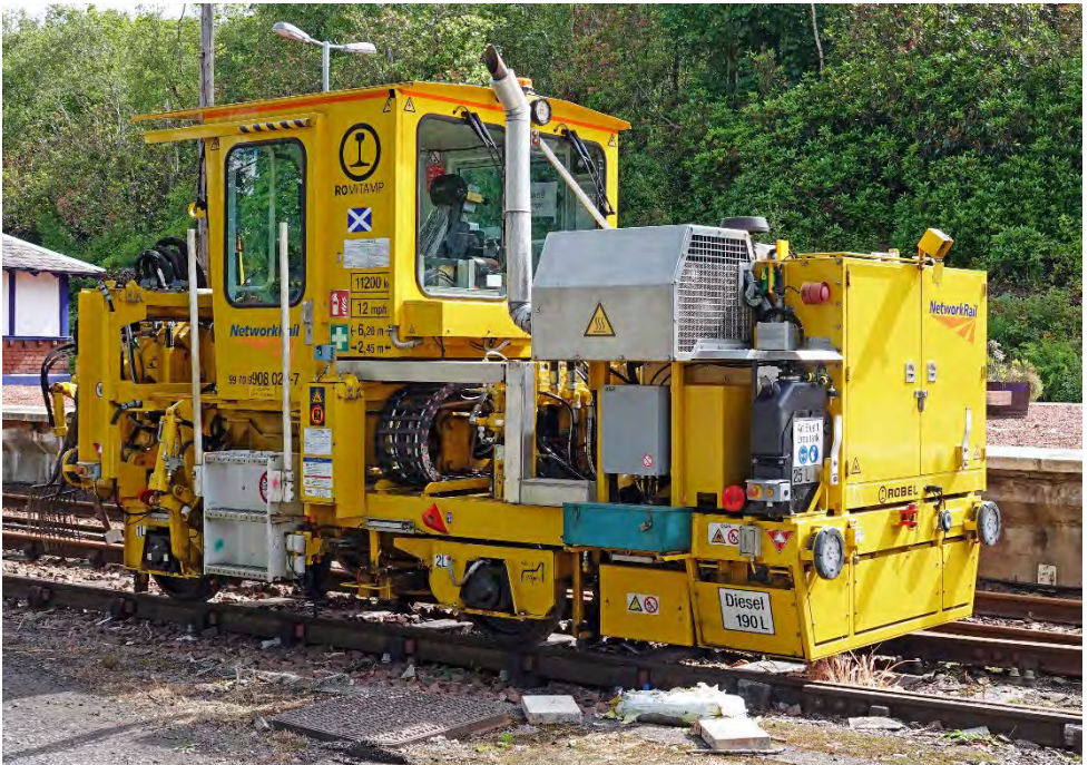
above & below Robel ROMITAMP GWS75 Mini-Tamper 99.70.9908.021-7 Garelochhead (10.40) 6 th July 2024 (TR) the other one in this class of two was shown on p73 in the Nov 2022 issue
