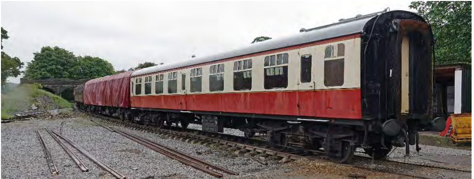
Two BR Mk1 TSOs 4215, 4844 recently arrived from SRPS, Bo'ness. 4844 is stripped out to be re-floored and will be modified to accept wheelchairs with double doors at one end.
