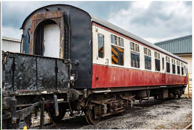
53 years since it entered preservation and 15 years since it was donated to a private owner based at EMB, North Eastern Railway Driving Trailer Third 8 Compartment 3453, built York Works in 1904, has been superbly restored to working order. Donated to the 1903 Autocar Trust in 2023 to operate with NER 3170 Autocar, it was launched on the 25 th May 2024.
