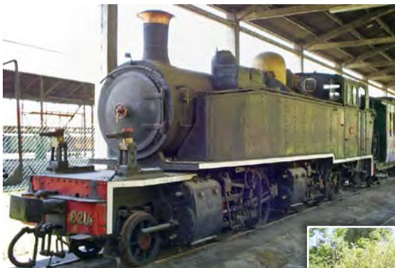
above E214 restored in a compound adjacent to the station, Regua, clearly showing the additional cylinders mid body
