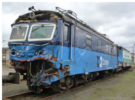
122023 has been in a major accident, probably with 122019 to which it is coupled as both cabs are damaged at that point, Usti Nad Laben shed, 11 th April 2017
