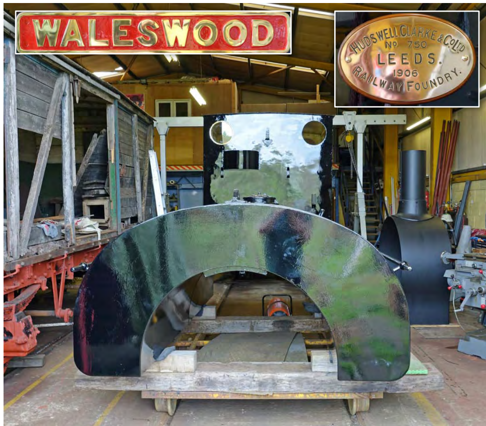
above [750] with saddletank to the fore, smokebox to the right and van 3224 to the left
