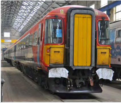
above 442424 with jumper cable covers in place, not something seen when in service 23 rd Jan
