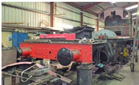
2-6-2T 5539, Llangollen, 8 th June 2014 being re-built from Barry scrapyard condition
