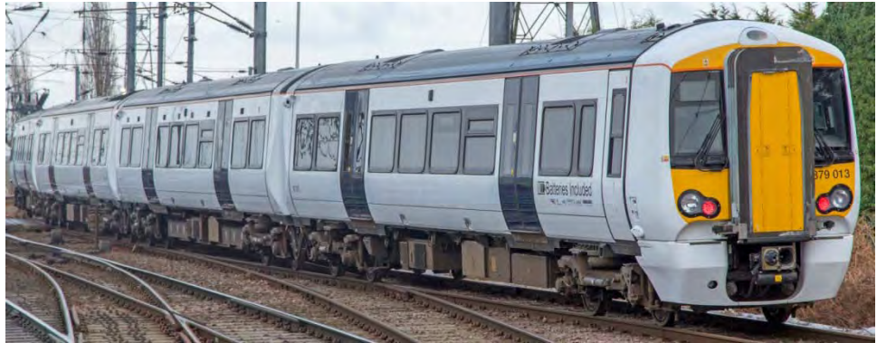
379013 converted to run on battery power (as the branding says shown below) as part of a NR / Bombardier project to trial battery technology is seen conducting testing on the Harwich branch, Manningtree, 6 th January 2015 (Colin James)
