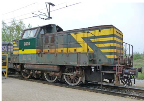
withdrawn 7404 at Antwerp Nord works with two new wheelsets and newly painted cab number, possibly saved for further use, 17 th April 2011
