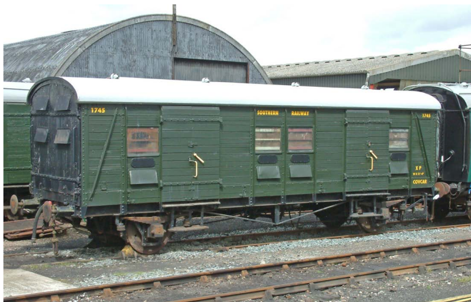
ex SR 4wCCT 1745 built at Eastleigh Works in 1938 Tenterden Town, Kent & East Sussex Railway, 11 April 2008
