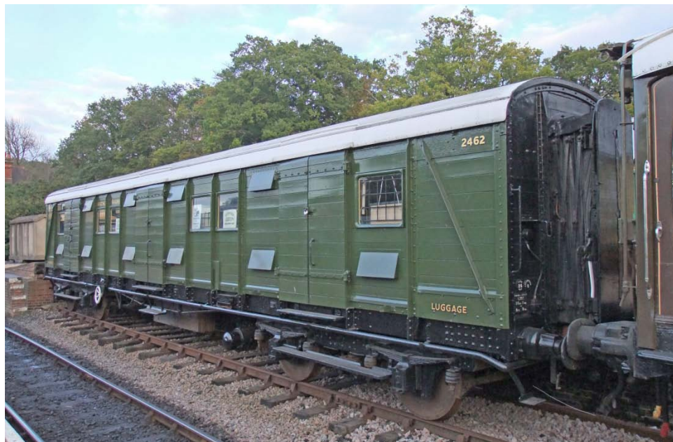
ex SR bogie luggage van 1745 with gangway connections built at Ashford Works in 1931 Horsted Keynes, Bluebell Railway, 22 October 2010
