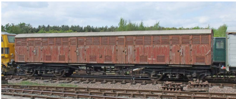
ex GWR design bogie Siphon G milk van W1025 built post nationalisation at Swindon Works in 1952 Ruddington, Nottingham Heritage Centre, 15 May 2010
