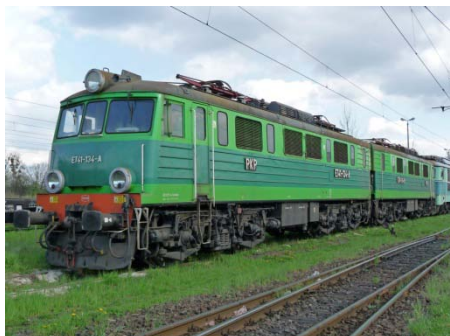
PKP have 3 classes of single cab Bo-Bo + Bo-Bo double locos, ET40, ET41 & ET42 which are used on heavy freights above is ET41 134-A + 134-B weighing in at a total of 167 tonnes, Wroclaw Głowny, 22 April 2010
